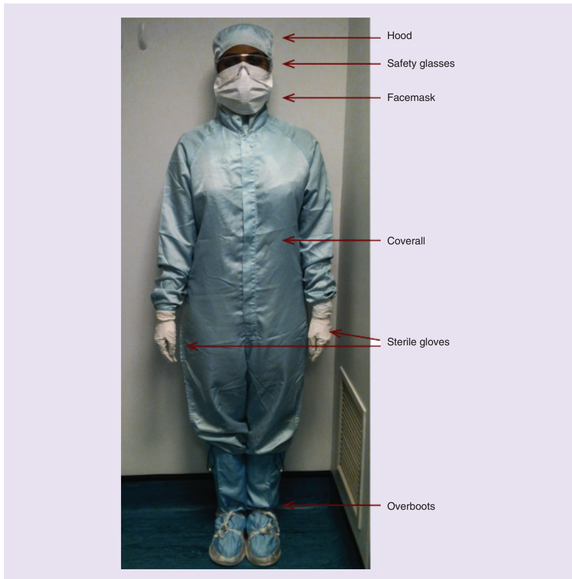
Figure 3. Garments required to operate/process at or above grade B. Operators are required to remove outdoor shoes and clothes and change into cleanroom tunics, trousers and clogs, and the donning of gloves and a mobcap (not shown above) prior to entering the facility. A second level of gowning is then performed prior to the operator moving to the grade B laboratories, this involves putting on fresh gloves, a hood, safety glasses, a face mask, coverall and overboots, all of these items will have been sterilized by irradiation.
